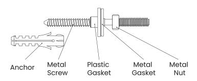
**2d.** Place the basin in position against the wall. Locating the fixing bolts through the holes in the rear of the basin. Push a plastic washer followed by a metal washer, onto each fixing bolt.
