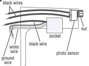
Take either black wire from photo sensor & place evenly against black wire from socket. Do not twist wires together before using wire connector. Fit a wire connector over the wires & screw the connector clockwise until you feel a firmness. Try gently to pull connector off the wires. If you can, pull off and repeat above steps until you have a firm connection.
