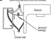
CONNECT THE WIRES, NOTE: Attach black fixture wire to black supply wire, white fixture wire to white supply wire. Do not mix them up. Use wire connectors (not provided). Connect bare fixture ground wire(s) to ground wire from outlet box. NEVER CON-NECT GROUND WIRE TO BLACK OR WHITE POWER SUPPLY WIRES.
