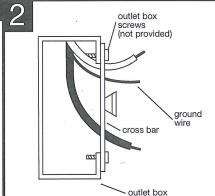
ATTACH cross bar to outlet box with outlet box screws (not provided).
