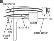
Take either black wire from photo sensor & place evenly against black wire from socket. Do not twist wires together before using wire connector. Fit a wire connector over the wires & screw the connector clockwise until you feel a firmness. Try gently to pull connector off the wires. If you can, pull off and repeat above steps until you have a firm connection.
