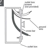
ATTACH cross bar to outlet box with outlet box screws (not provided).
