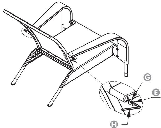
**3** Attach the **Seat D** to the **Seat Back A** using 3 **Bolts F** with **Washers G**, inserted through the **Seat** and into the **Seat Back**. Tighten using the **Hex Wrench H**.
