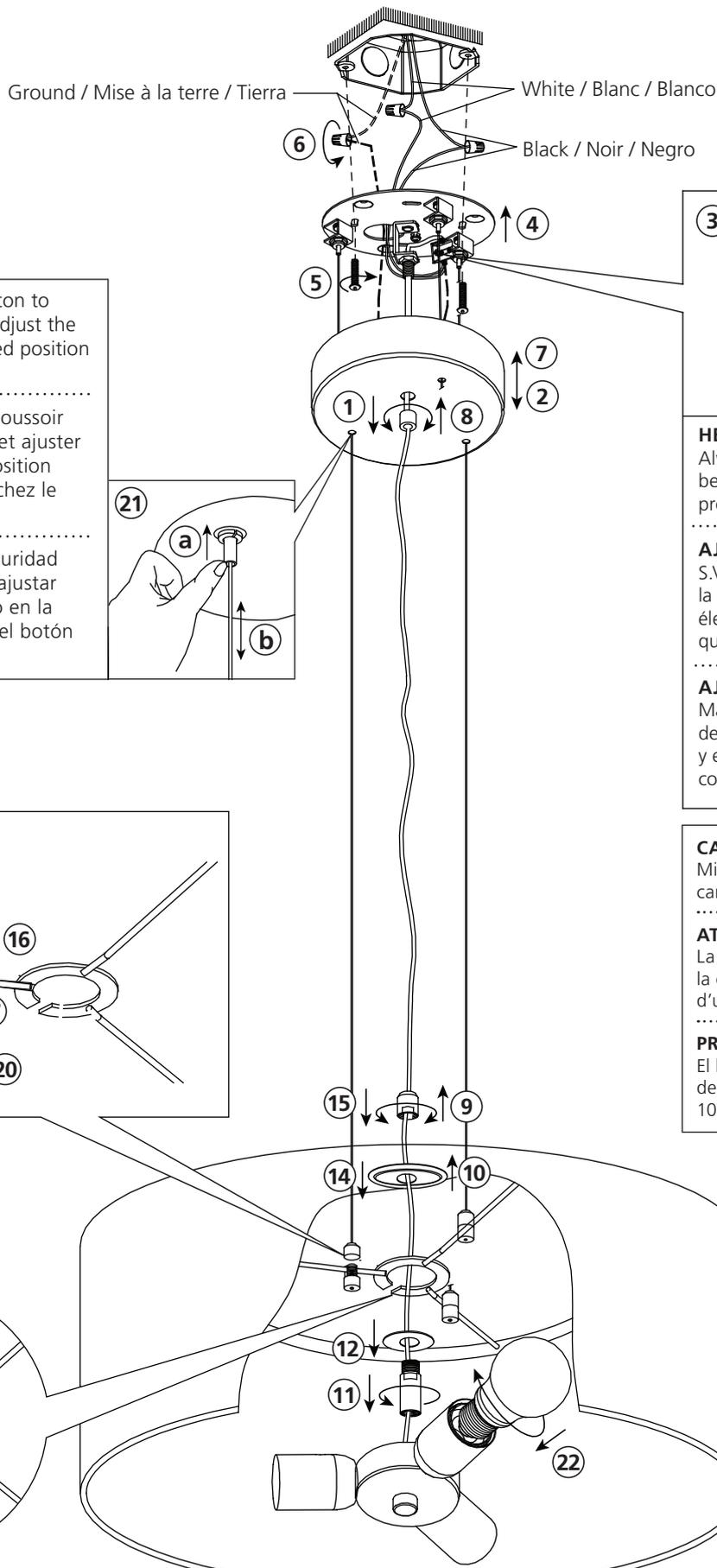
Push the "push-pin" button to release the tension and adjust the height. Once set in desired position release the push pin.
