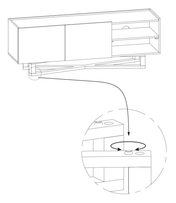
Note: Levelers on the bottom of the legs can be adjusted if floor is uneven.
