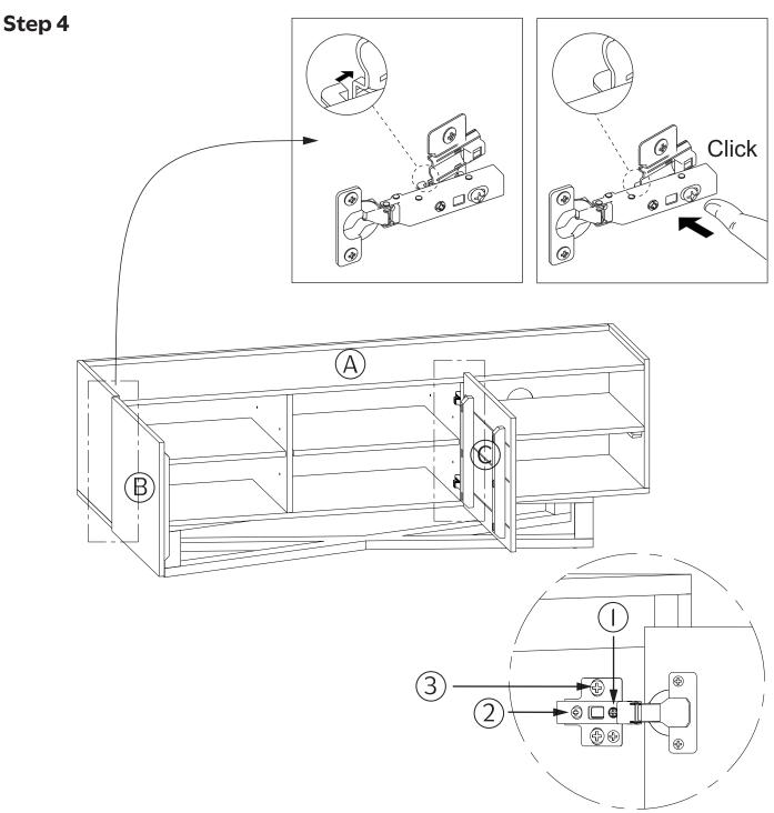
Attach Doors B and C using adjustable hinges on Top A.
