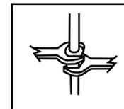
Tighten connection with two wrench to prevent damage to tube body. Be careful not to bend the stem as this will void the product warranty.
