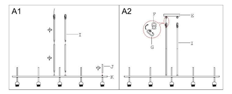
Step A1 » 1) Carefully pass the fixture wires through one side of tubes (I) and loops (F).
