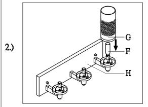
Step.2: Place the candle tube(F) and glass (G) on the socket
