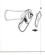
water and relieve pressure! Detach handle button small flathead screwdriver, unscrew set screw lien Wrench and take off handle.
