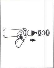
Remove handles. Unscrew Dome Cap counter clockwise by hand. Unscrew Retaining Nut using adjustable wrench, take out cartridge assembly and inspect. Replace parts as necessary. Reassemble parts by reversing steps.
