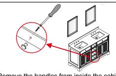
® Remove the handles from inside the cabinet doors and drawers and reinstall on the outside. Do not over tighten when reattaching.
