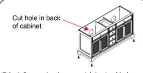
Installer must cut appropriately sized hole in back of cabinet to accomodate existing placement of hot & cold wall valves & drains.
