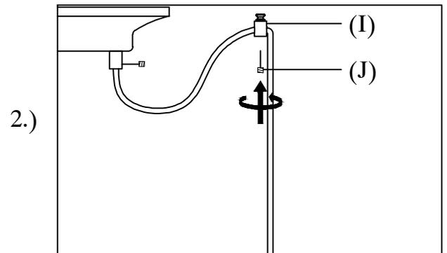
Step2 :Adjust wire length to desired mounting height, and tighten strain relief screws to secure.
