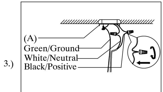
Step3 :Wire fixture to wires in outlet box. Green wire is for Ground.
