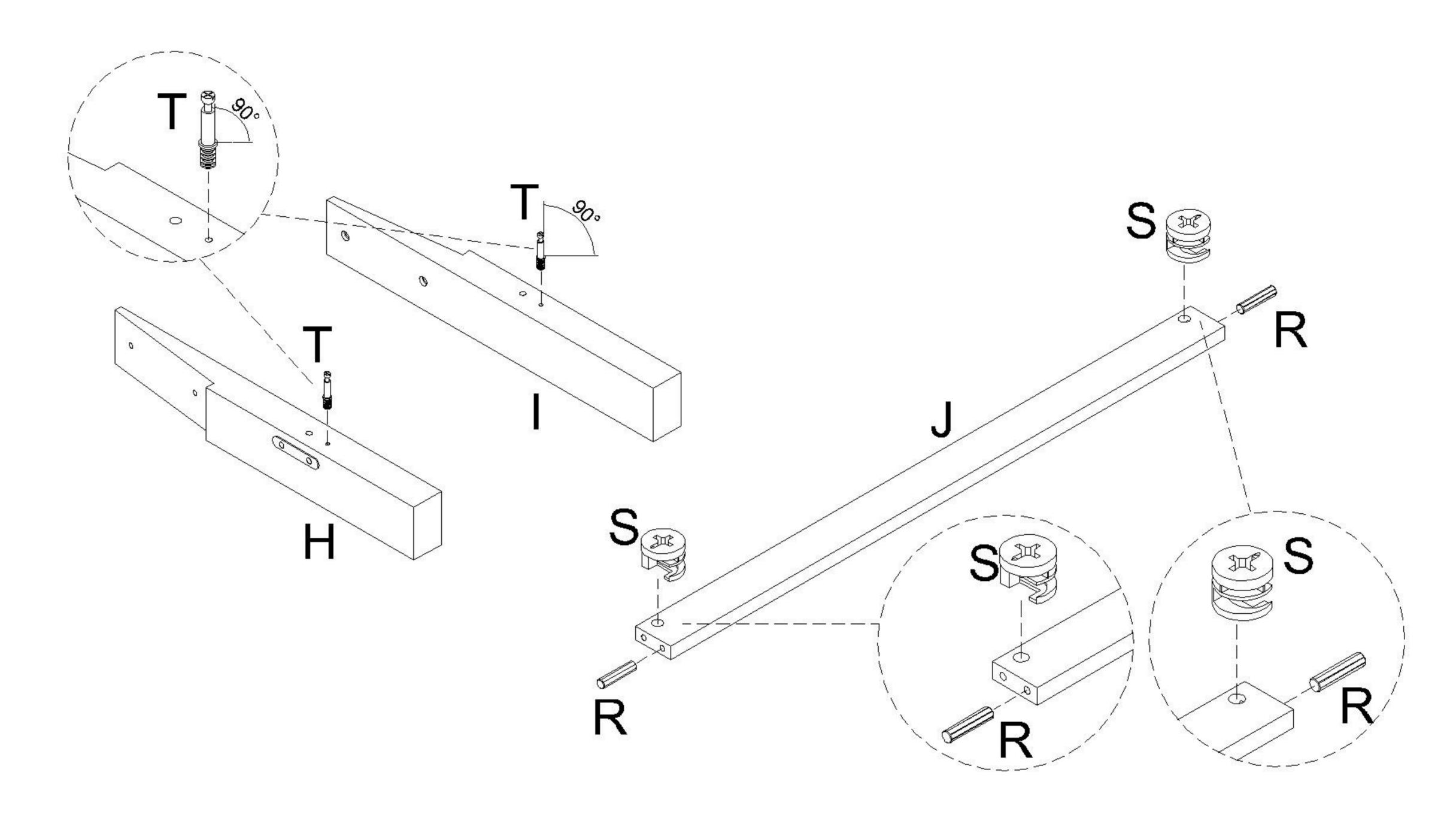
2 Attach Left & Right Headboard Post (H & I) to Headboard Bar (J) and secure with Cam Lock (S). Cover Cam Lock (S) with Cam Lock Cover (U).
