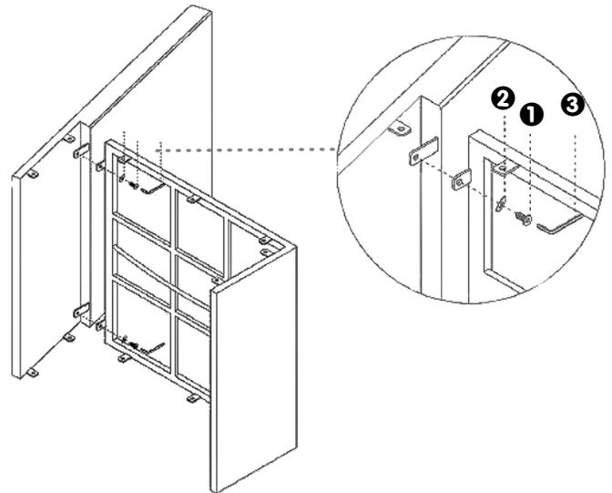
**2** Place the **Left Side Panel C** open-side up on a flat surface, then align the **Backrest/Seat** on top as shown. Align the eyelets on both pieces, then insert a **Bolt 1** with **Washer 2** into each of the 6 aligned sets of eyelets.
