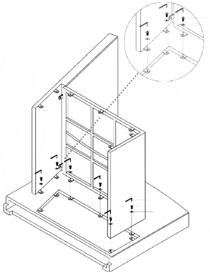
**3** Locate the **Right Side Panel** **B** and lay it on a flat surface with the open side facing up. Position the partially-assembled chair on top of the **Right Side Panel** as shown. Align the eyelets on both pieces, then insert a Bolt **1** with Washer **2** into each of the 6 aligned sets of eyelets.
