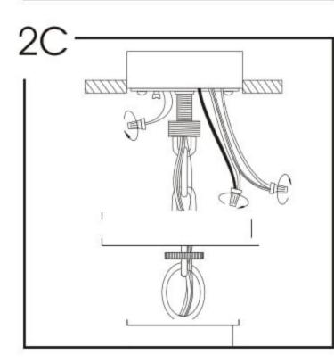
Strip 3/4" of insulation from wire ends. Connect house ground wire to fixture ground wire. Twist wires together using wire nut. Connect the black house wire to the smooth or black fixture wire. Twist wires together using wire nut. Connect the white house wire to the ribbed or white fixture wire. Twist wires together using wire nut.
