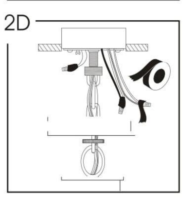
Tape wires and wire nuts together using electrical tape.
