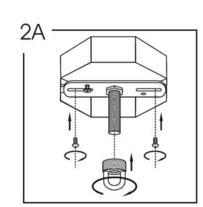
Screw crossbar assembly into junction box using outlet box screws. Thread screw collar onto threads of crossbar assembly.
