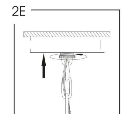
Carefully tuck wires into junction box and secure canopy to ceiling using screw collar ring.
