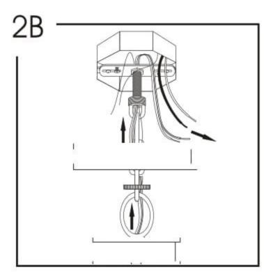
Slip screw collar ring and canopy onto chain, and hang fixture onto screw collar using an open link of chain. Close link. Thread wire and ground cable through screw collar ring, canopy, chain, screw collar, and through threaded tube on crossbar assembly. Pull wires through.
