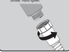
Thread Bracket onto shower arm by turning it in a clockwise direction. Tighten with adjustable wrench
