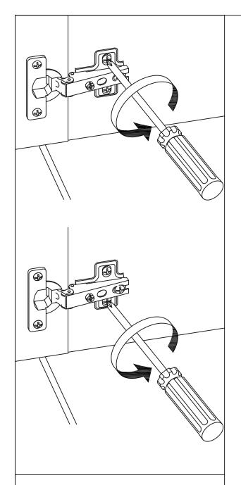
**STEP 15.1.** IF THE GAP ON THE TOP OR BOTTOM ARE NOT BALANCED, LOOSEN BOTH HINGE BASE SCREWS.
