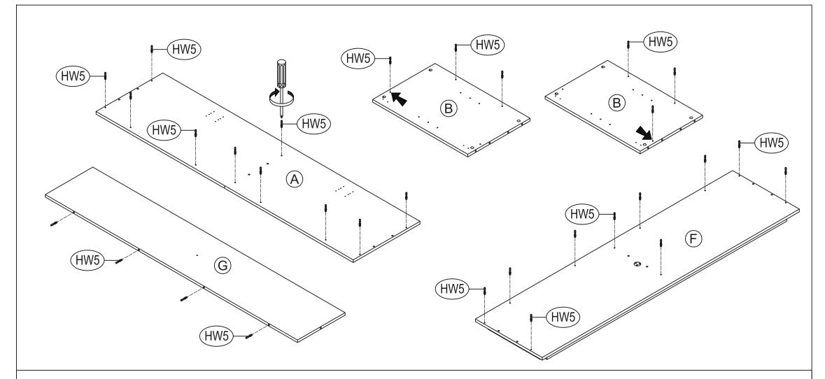
STEP 1 ATTACH CAMBOLTS (HW5) TO TOP PANEL (A), SIDE PANELS (B), BOTTOM ASSEMBLY (F) AND UPPER BACK PANEL (G).
