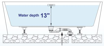
Anti- leak drain and pipe
