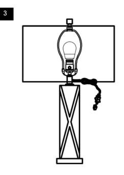
Step2 Insert the bulb(G) into the socket(C).
