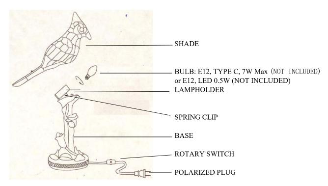
**Note**: 1. The diagram illustrates the installation of your new luminaire.
