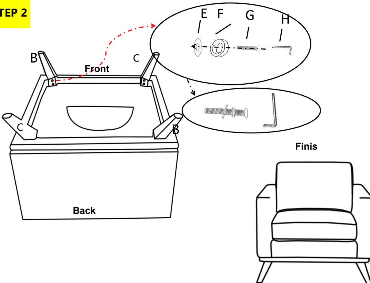
***NOTE: DO NOT TIGHTEN ANY BOLTS UNTIL ALL BOLTS HAVE BEEN STARTED!***
