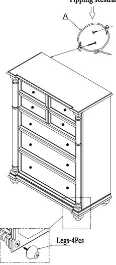
Adjust Leveler if needed to level case on uneven floor.
