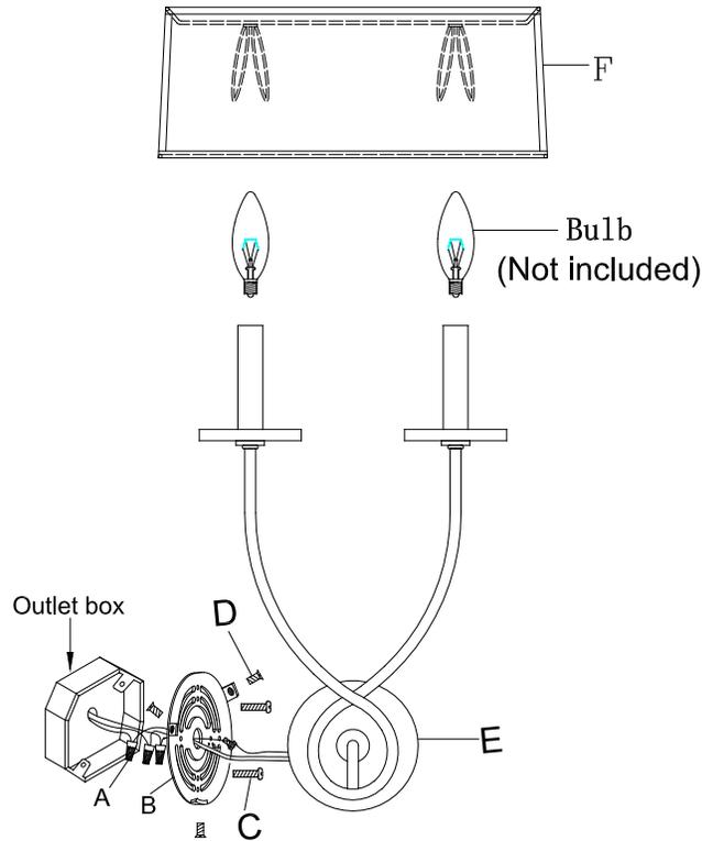
1. Carefully remove the mounting plate (B) from the back plate(E) by removing side screws(D).
