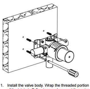
of the joints in Teflon tape and connect the water inlet and outlet.
