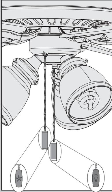
The fan pull chain controls the speed: from high to off.
