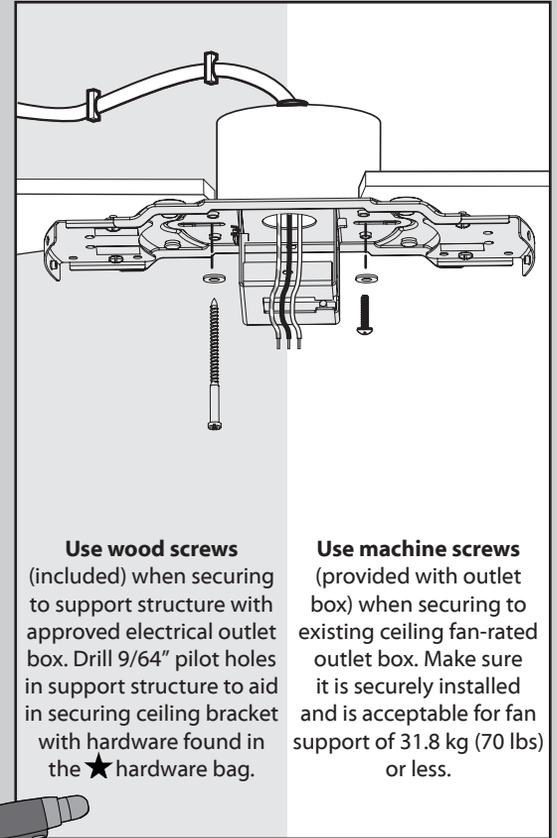
**Use wood screws** (included) when securing to support structure with approved electrical outlet box. Drill 9/64" pilot holes in support structure to aid in securing ceiling bracket with hardware found in the ★ hardware bag.
