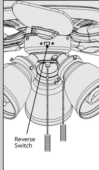
To switch the direction of air flow, move the reverse switch to the opposite position.
