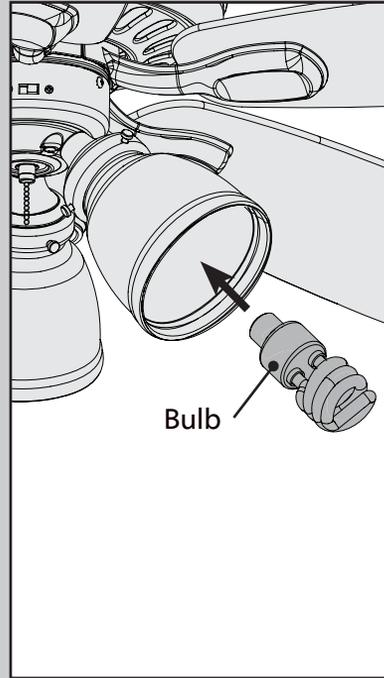
Install a bulb into each of the sockets. When necessary, replace with bulbs of the same wattage.
