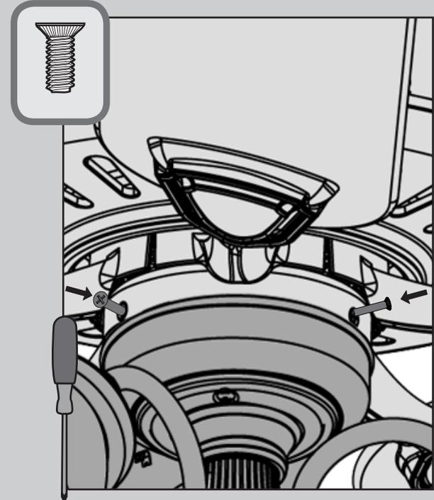
⊗ Insert three switch housing screws found in the ☰ hardware bag.
