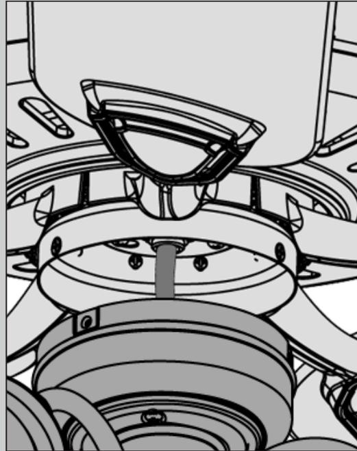
Lift the lower switch housing up until the holes line up with the screw holes in the upper switch housing.
