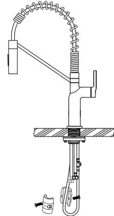
Connect pullout hose to quick connect and insert weight (loose-install).
