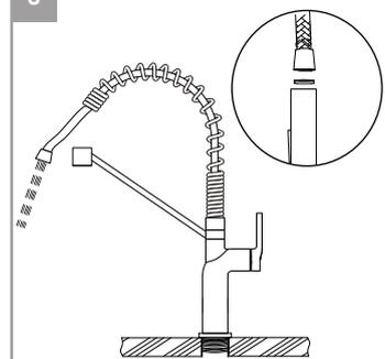
Unscrew spray head by hand. Hold the tip of the spray hose down and turn on the faucet and let the water run 60 seconds to flush any debris, the re-connect spray head. Ensure gasket is present.
