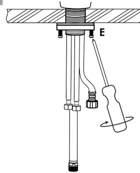
Slide washer and thread the mounting nut onto threaded shroud. Turn faucet to desired handle position. Securely tighten clamp screws (E).
