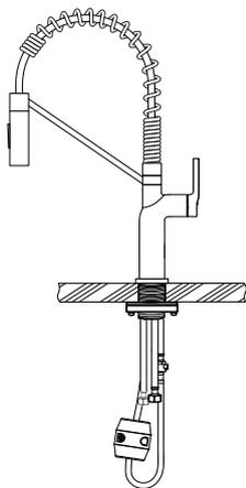
Secure weight on lowest vertical point on pull-out hose side. (not on quick connect side).
