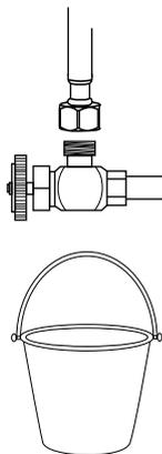
Before connecting supply hose, flush supply valves to clear any debris. Place a bucket underneath valves and run water for 5 to 10 seconds. Turn water off.
