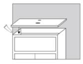
perimeter of the vanity body. With assistance from another person, slowly and carefully set the counter top onto the vanity cabinet. Once positioned, press firmly into place.
