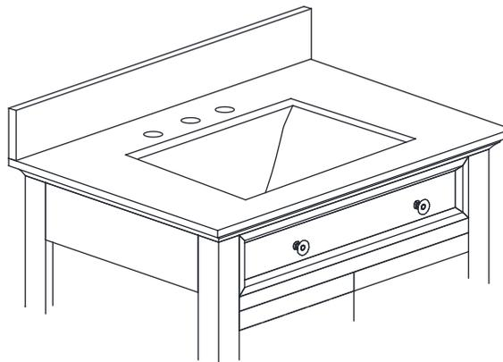
Finally, place the bottom side of back splash with sealant onto the countertop and check alignment of back splash. Adjust the leg levelers as needed
