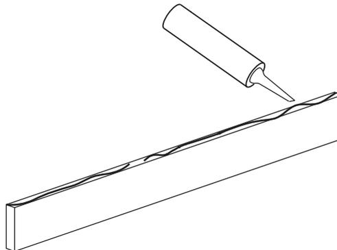
Apply silicone sealant evenly along the bottom and backside of back splash.
