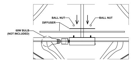
STEP 3: Install the bulb, do not use bulb that exceed 60watts.
