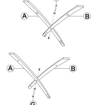
NOTE: Ensure the metal tab on Leg B faces inward, as shown in the top drawing.
