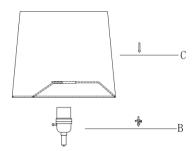
Step 4. Gently screw the bulb (D) on the socket (B).
