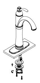
From underneath the sink,replace mounting hardware assembly. Tighten lock nut to secure the body.
