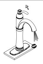
After installing faucet, remove aerator and turn on water to remove any left of debris.
