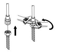
Apply pipe tape on threads of the inlet port. Tighten end of shank with wrench and slip hose into the inlet port.
