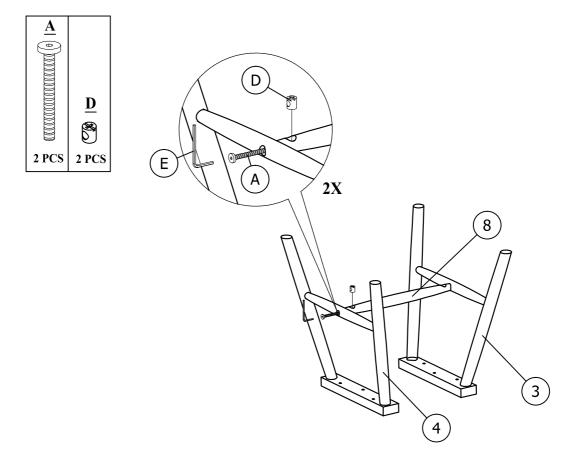
DO NOT TIGHTEN BOLT COMPLETELY.
