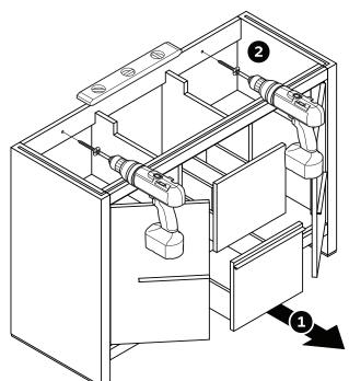
*IMPORTANT:* Consult an expert for the proper screws/bolts to use when attaching to various constructions. Screws provided <u>do not</u> attach to all wall construction types. Anchors are not required if brackets are installed in stud.
