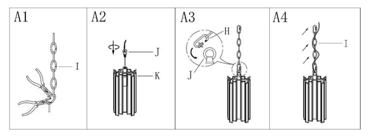
*Step A1* » By measuring, determine the correct number of links needed for proper hanging height. Using the chain pliers, disconnect and discard the unwanted part.
