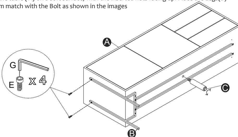
**Step 2:** Attach the leg using the Bolts D, E and F and Allen Key (G) provided
