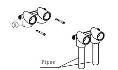
3. Connect G1/2 connector to Inwall Body with PTFE tape, ensure connector outside the wall no leakage and keep in horizontal level.
