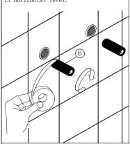
4.Unscrew the seven M4 screws with Allen Key, Slip out the wall cover No.2 and then put out the Backcover No.3.
