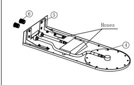
7. Install Backcover No. 3 with M4 screw and then install wall cover No. 2.
