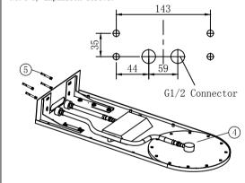
$6.\,\mathrm{Tighten}$  screws No. 5, connect two hoses to G1/2 connector No. 6 and guaratee no leakage. Cut the end of PTFE taped connector by cutting machine if need to make connector shorter and repeat installation from step 3.
