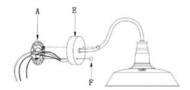
Attach the mounting plate assembly(A) to outlet box with mounting screws (C).
