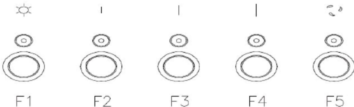
**Function Button:** LED light button F1 low speed F2 medium speed F3 high speed F4 time-delay/on-off F5
