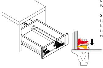
Unlatching the drawer and removing it from the runners is just as easy.
