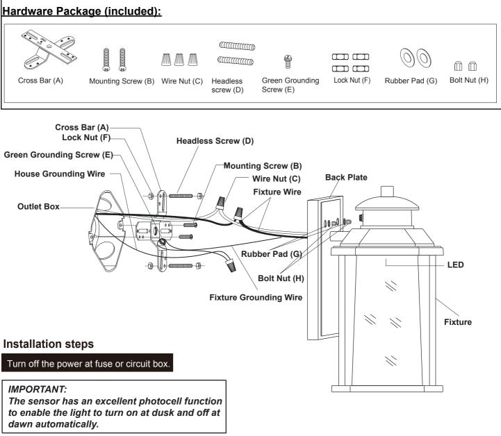
1. Attach the headless screws to the cross bar, then secure it with lock nuts.
