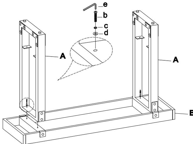
Step 2. Loosely attach bottom shelf (C) to the each leg frame (A) as show below. Securely tighten all bolts with Allen wrench (e) .
