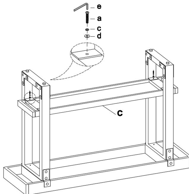
Step 3. Turn the assembled table to an upright position. Securely tighten all the bolts with Allen wrench (d). Assembly is complete.
