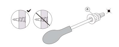
**Stud Mounting**(2b)Using a stud finder, locate and carefully mark the location of studs on the wall where you want to hang your shelf.
