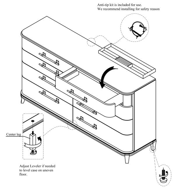
Adjust Leveler if needed to level case on uneven floor.
