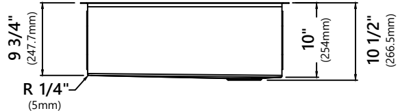
Model #: KWU110-28 Sink Dimensions: 28" x 19" x 10" Min Cabinet Size: 30"
