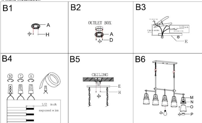
Step B1 » Unscrew knob nuts (H) from mounting plate (A).
