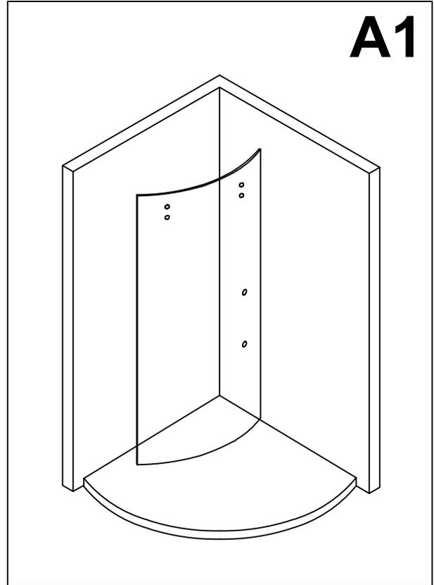
2. Arrange the glass according to the configuration you've chosen from page 4. Measure \*71 1/4" from the floor or curb of base. Mark this location. This will be the height of the center of your wall mount bracket assembly (#1). Measure \*32 7/8" out from the corner for the VG6031CL36 or \*35 3/8" for the VG6031CL40. This will be the center point of your wall mount bracket assembly.
