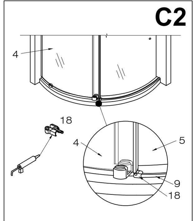
3. Screw the door threshold clip (#18) to the base curb or floor using the 1 1/8" phillips screw (#15). Silicone the screw cap to the threshold clip (#18).
