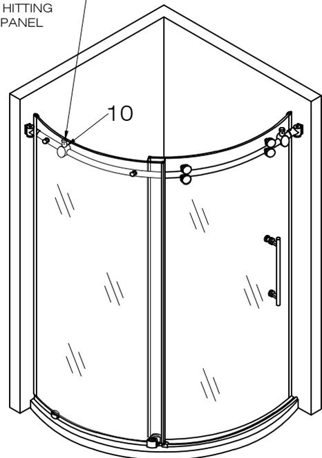
**E. INSTALLING THE WATER SEAL STRIP**
