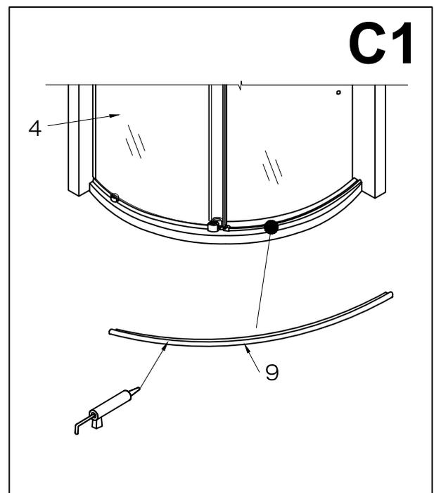
2. Apply silicone to the threshold clip (#18), slide on to the fixed panel and place on the threshold (#9) as needed.
