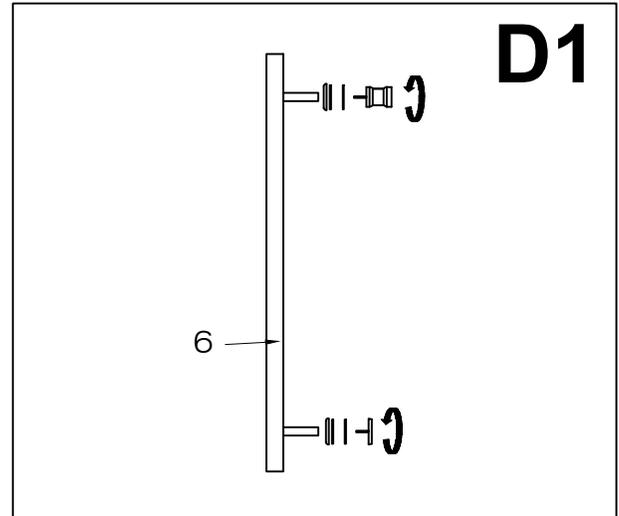
2. Place the handle to the position on the door. Place plastic washers (supplied) on each side of the door.
