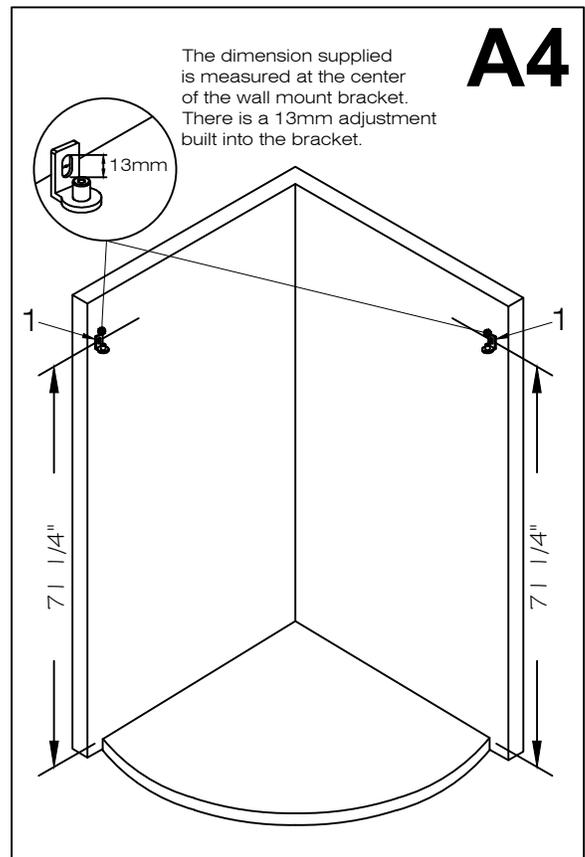
5. Drill holes and place plastic anchors (#17) inside them. **⚠ Preferred method of installation negates anchors and has the installation going right into studs.**
