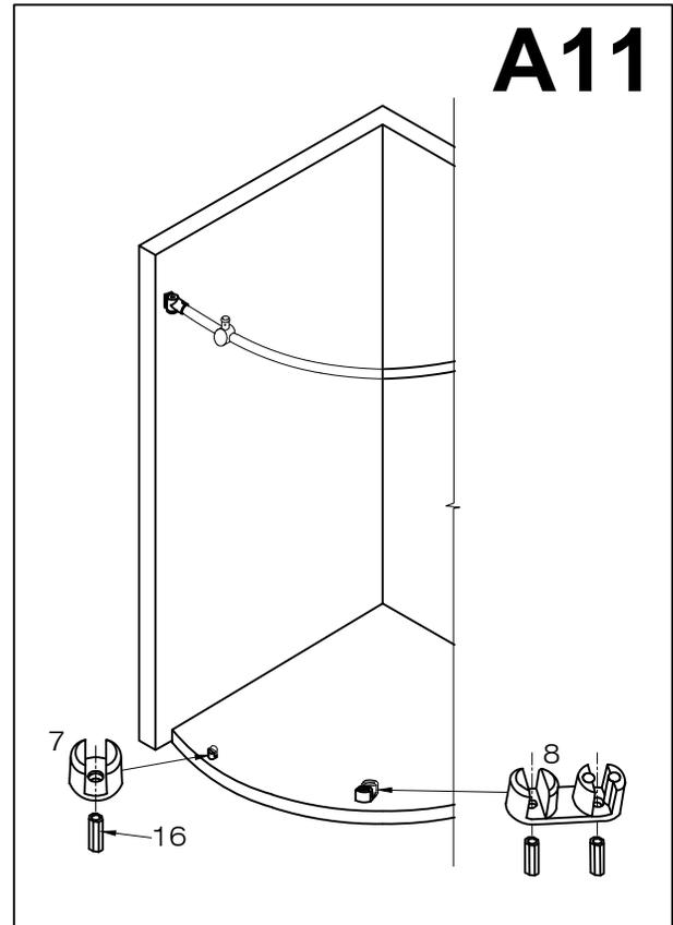
12. Screw in the fixed panel bottom clip (#7) and the door bottom guide (#8) to the floor with 1 1/8" screws (#15).
