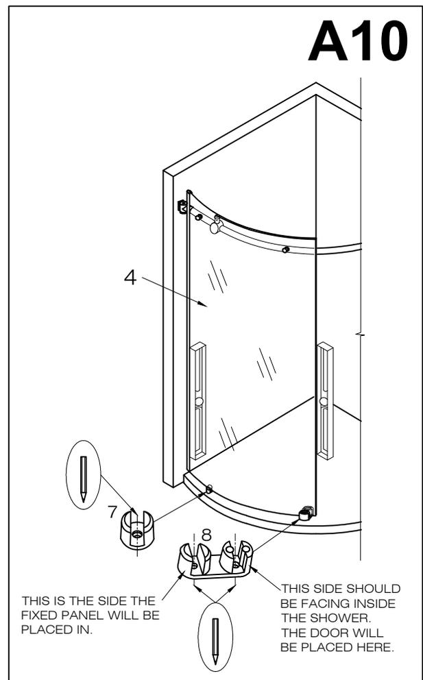
11. Remove the front fixed panel (#4) from the position in the opening. Drill holes where you marked your locations for the fixed panel bottom clip (#7) and bottom door guide (#8) and place the plastic anchors (#16) inside them.
