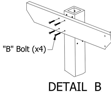
**9)** Lift an Upper Support Beam into Place as Shown. Support One End of the Beam Until Step 10, and Secure the Other End to the Arch Assembly from the Previous Step Using (4) "B" Bolts, as Shown in Detail "A".
