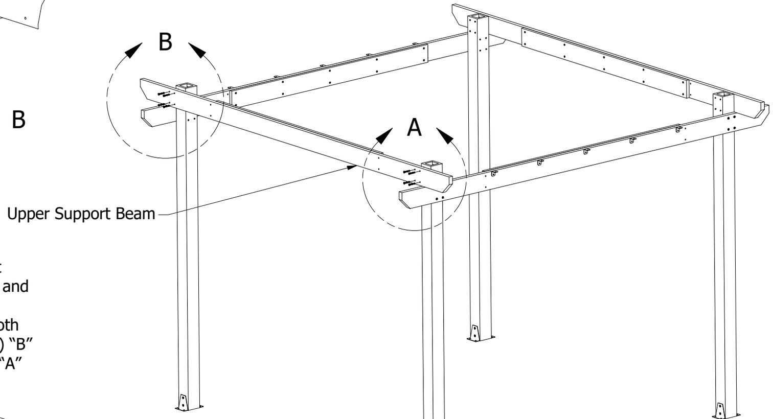
**13)** Lift an Upper Support Beam into Place as Shown and Set on Top of the Lower Support Beams. Secure Both Ends to the Posts Using (8) "B" Bolts, as Shown in Details "A" and "B".
