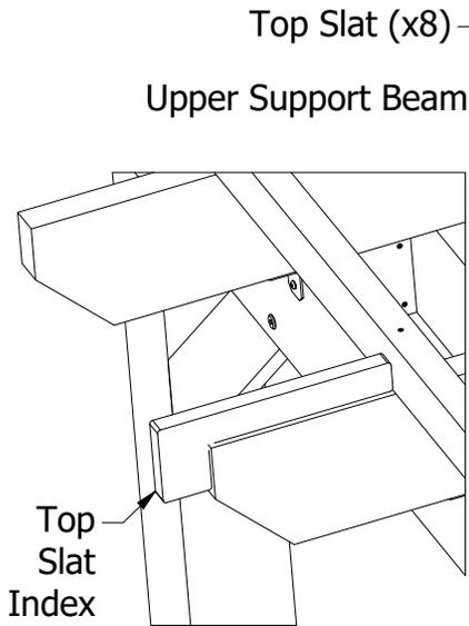
**29)** Use the Top Slat Index to Set the Location of the First Top Slat. Set the Top Slat Index on Top of the Joist as Shown Above, and Adjust the Top Slat Until it Rests Against the Top Slat Index.
