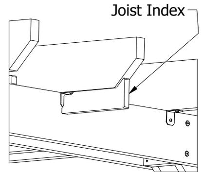
**26)** Use the Joist Index to Set the Distance Each Joist Overhangs the Lower Support Beam. Place the Joist Index Against the Lower Support Beam as Shown and Slide the Joist Until the 45° Cut Rests Against the Joist Index.
