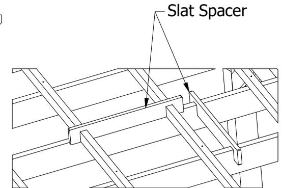
**31)** To Set the Location of Each Subsequent Top Slat, Use the Slat Spacer to Set the Center-to-Center Distance Between Top Slats. Use the Second Slat Spacer to Maintain Proper Spacing of the Joists as Shown Above. Move Each of the Spacers Accordingly so they are Near the Area of the Top Slat Being Secured. This will Ensure all Slats Remain Straight and Square with One Another.
