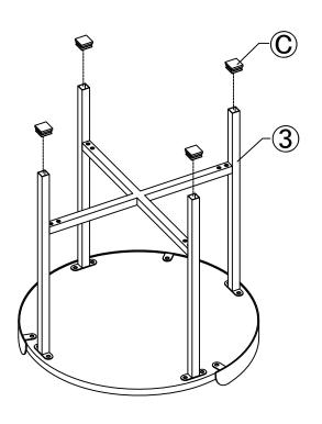
$\ensuremath{^{**}}\xspace$  Attention: Use the carton as a working surface to prevent table-top damage during assembly.
