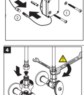
Install the adapters and filters on the stops.
