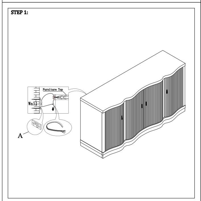
The Anti-tipping HW is attached at the upper right back of the server, please remove it for assembly.
